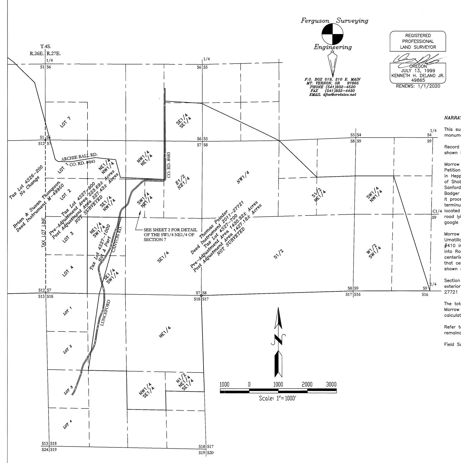
PROPOSED PROPERTY LINE ADJUSTMENT SITUATED IN THE SW1/4 NE1/4 OF SECTION 7, T.4S., R.27E., W.M. MORROW COUNTY, OREGON Completed on March 13, 2019 Sheet 1 of 2
