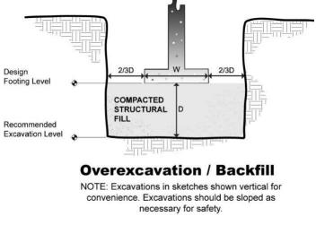
Special care must be taken with site soils to maintain proper moisture conditions. Over wetting of soils being placed may result in underlying soils exceeding their optimum moisture condition resulting in "pumping" during earthwork activities. If such conditions occur, over excavation, moisture conditioning, and recompaction may be required.
