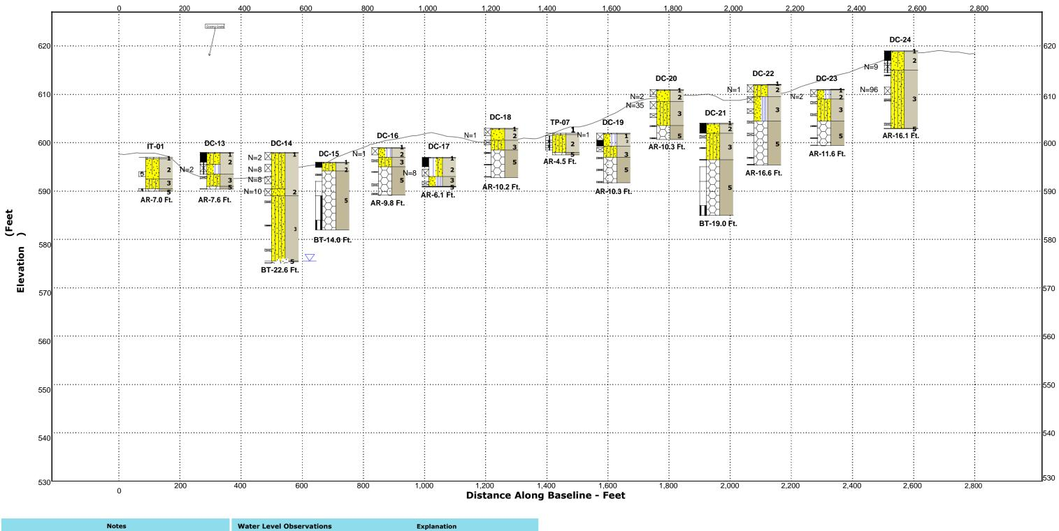
See Exploration Plan for orientation of soil profile. See General Notes in Supporting Information and GeoModelfor symbols and soil classifications. Borehole DC-13 Number Soils profile provided for illustration purposes only. Soils between borings may differ AR - Auger Refusal BT - Boring Termination Water Level Reading  $\boxtimes$  $\nabla$ Sampling-GeoModel Layer at time of drilling. Borehole Water Level Reading Lithology after drilling. Borehole AR Termination Type BT
