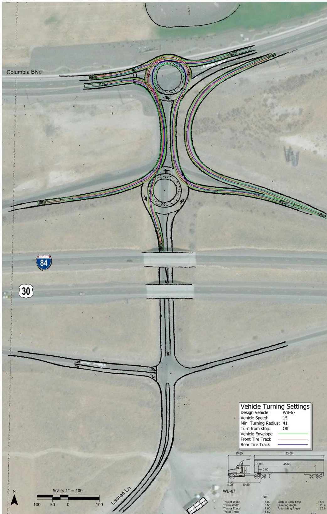
Figure 10 – Concept 'C2' Sketch Level Layout with WB-67 Design Vehicle
