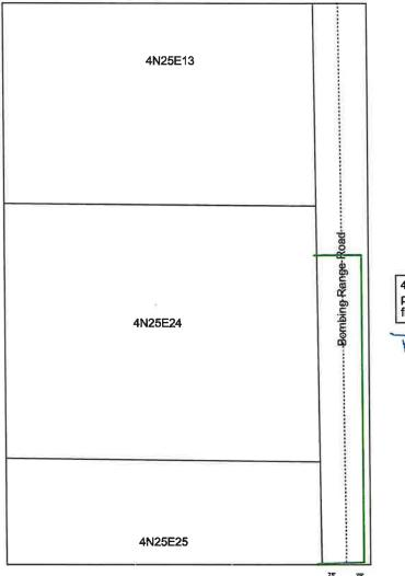
40 conduit fiber package, located 50' from centerline
